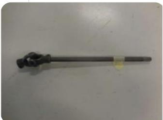
The removed shaft with U-joint.
