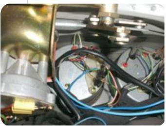
Reinstall the speedometer into the dash. Be sure that the wiper mechanism is not catching the wiring!
