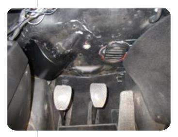
Use some selftapping screws to install this cover. Also apply some sealant before installing it!
