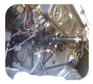
**STEP 11** Fit the top mounting clamp on the EZ column and fit the entire column in the car.
