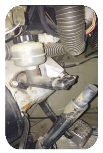
Install the EZ output plug into the original steering shaft. Before welding this, it is recommended to adjust it to the EZ-unit and weld it to this unit.
