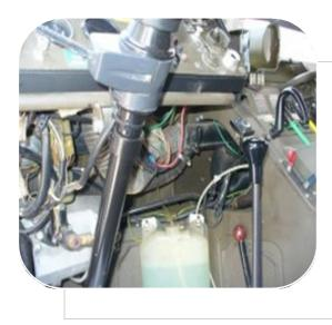
Remove the indicator switch and the steering wheel from the original steering column. Then remove the horn wire through the bottom of the original steering shaft. You will have to connect this to the sliding contact of the EZunit in a later step.
