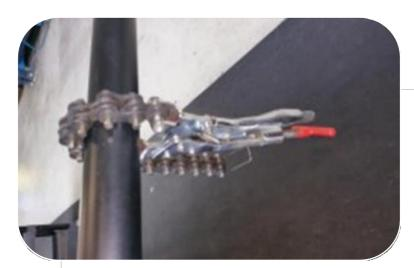
Use the pipe cutter to cut through the original steering tube. Use the EZ-unit to determine the right length.
