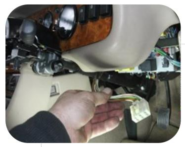
Step 5. Undo the two cables from the steering column.
