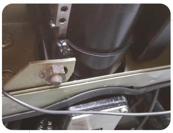
Step 17. Secure the input tube with the original clamp.
