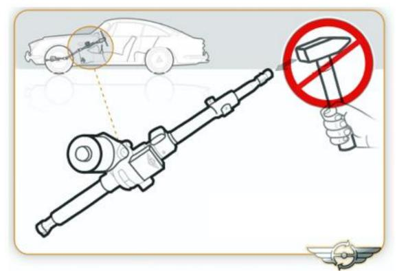
Never strike the input shaft with an object during or after assembly. This can adversely affect the sensors.
